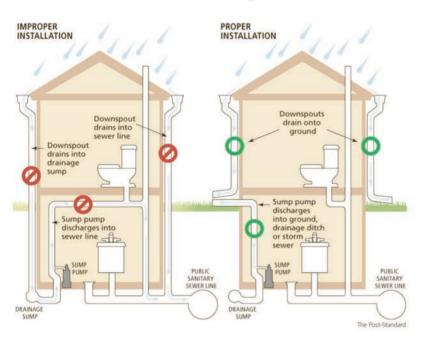
In some homes, sump pumps do not pump the water outside. Instead, they are connected into the sanitary sewer system. These types of connections are in violation of the Ontario Building Code and the Municipality of Central Huron's Sewer Use By-Law 39-2018. As well as a sump pump connection to the sanitary sewer can cause a back-up which will lead to flooding your basement with sewage! It is also detrimental to the operations at the Clinton Sewage Treatment Plant.
